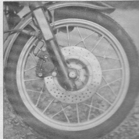
Valve too close to spoke for access
